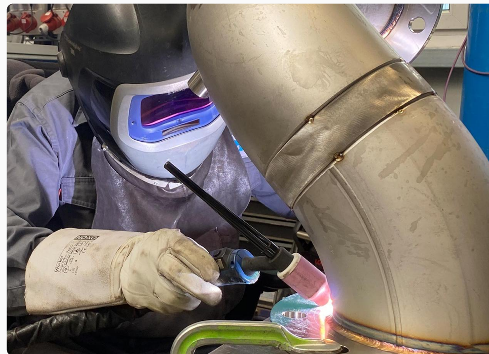
Stainless steel pipeline construction for a pumping station
