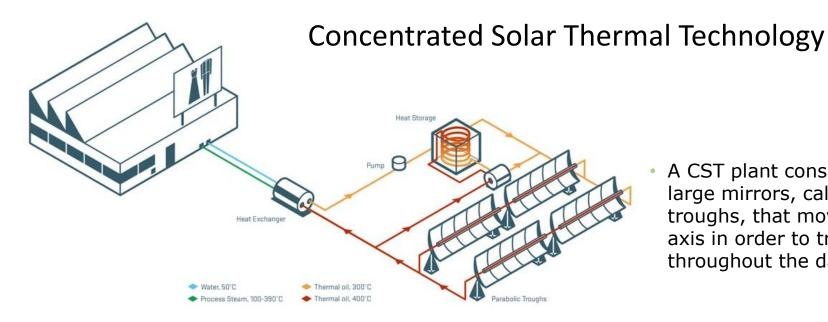
A CST plant consist of rows of large mirrors, called parabolic troughs, that move about one axis in order to track the sun throughout the day
